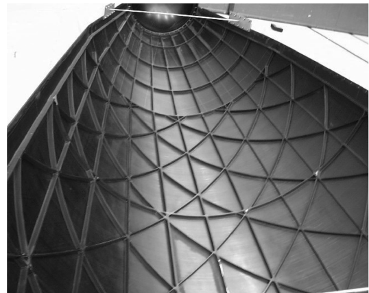
Fig. 5 Interior view of the Minotaur fairing half-shell.
