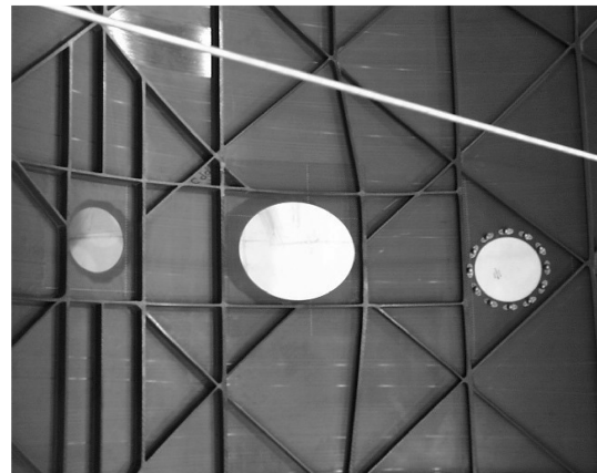
Fig. 6 Illustration of utility ports in the Minotaur fairing.
